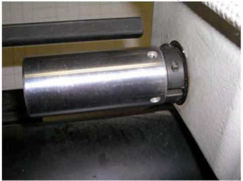
3. Loosen the 3/16" screw in clamping nut on back of headstock (thing next to handle)
