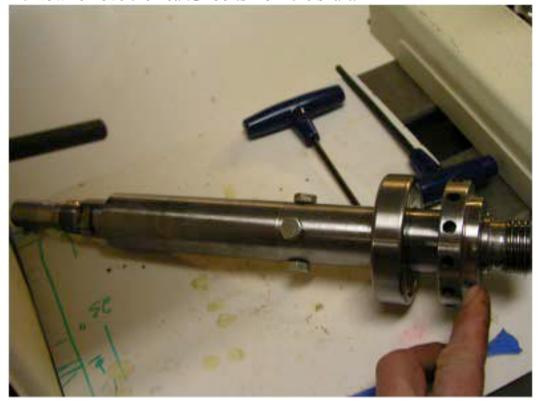
15. If you were lucky like me, the front bearing started to slide down the shaft as I banged it out. If not you will need to get it started down the shaft. A bearing splitter would be the easiest way, but you may find a flat head screwdriver with a few taps will work as well.
