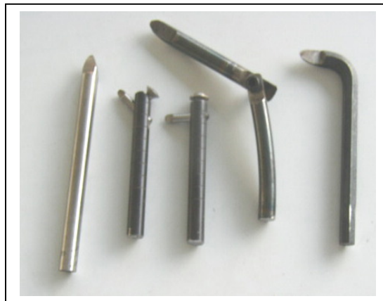
Tool Bits, Left to Right: 3/8" HSS Straight Bit, 3/8" Boring Bar with 3/16" HSS Bit, Ditto, 3/8" Drill Rod Adjustable Angle Bit (Source of Materials – ENCO), Ground Hex Wrench Bit
