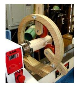
Here are some pictures of a (3) wheeled steady rest I made last month. The basis for the plans came from American Woodworker's website (imagine my surprise at something useful coming from there!). I tweaked the design a bit since I really didn't like their clamping mechanism. I also scaled the size up a bit to take advantage of my Jet lathe's increased capacity. (Well, you didn't expect me to just use their design as is, did you?)
